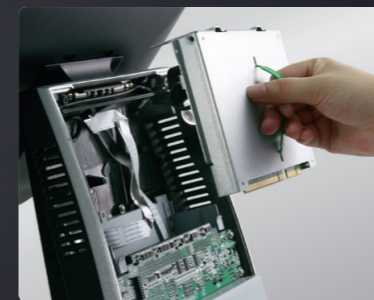
CPU module can be extracted for efficient upgrades and maintenance
